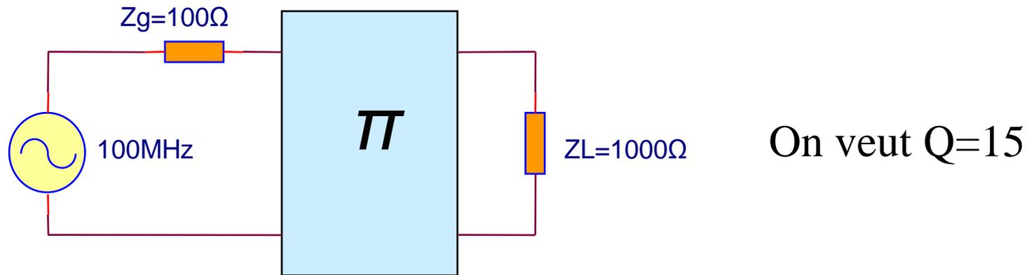
$$Q_L = \mp \sqrt{n-1} = \mp \sqrt{9} = \mp 3 \quad Q_\pi > Q_L \quad \text{faisable}$$
