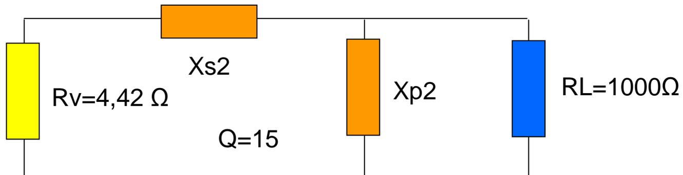
$$X_{P2} = R_P / Q_P = R_L / Q = 1000 / 15 = 66,7 \Omega$$
